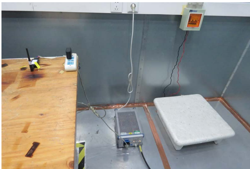
Picture 2: Conducted Emissions Test Setup
