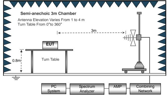
(C) Radiated Emission Test-Up Frequency Above 1GHz
