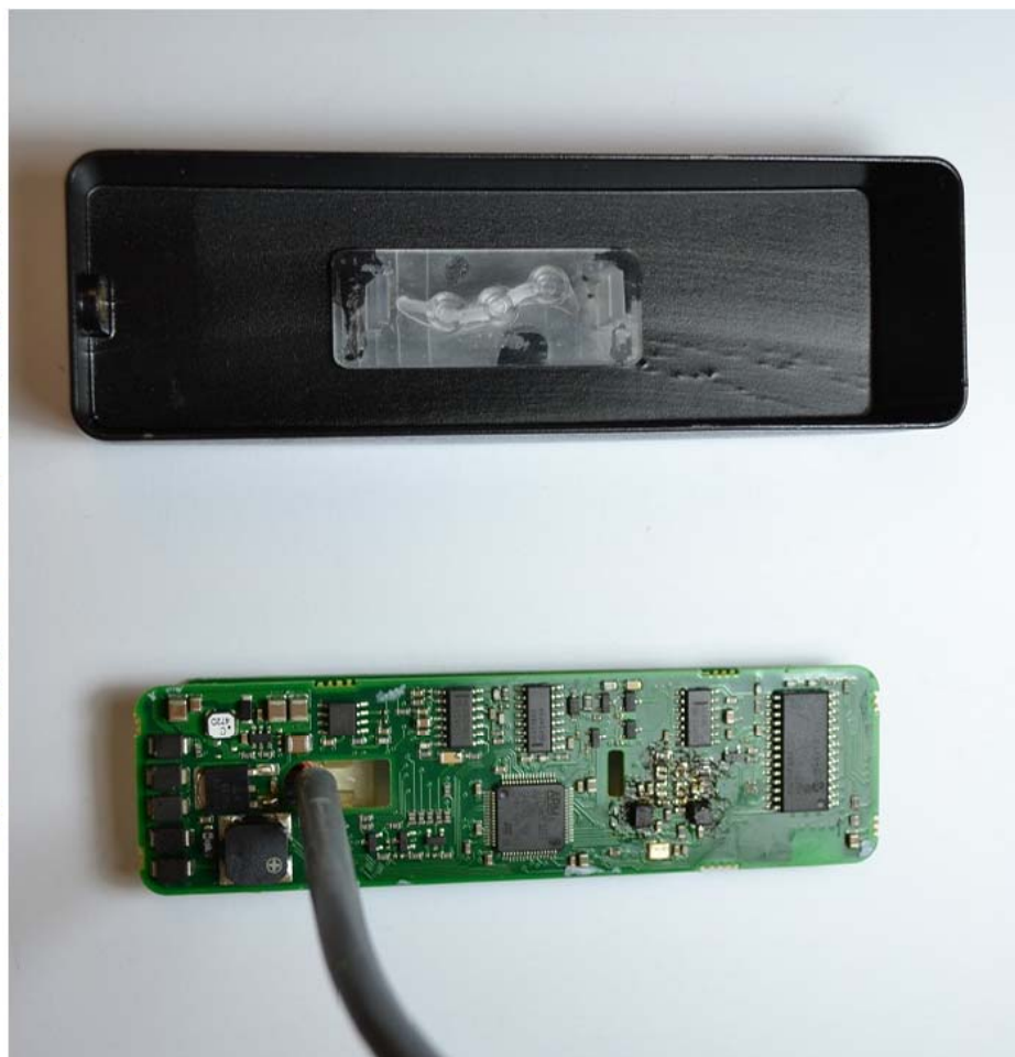
T15 Multi Tech - Front Cover and PCB Assembly
