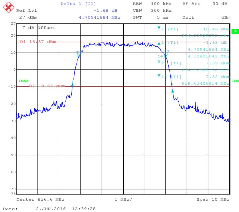
**PCS Band (Part 24E)****99% Occupied & 26 dB Emissions Bandwidth for GSM (GMSK) Mode**
