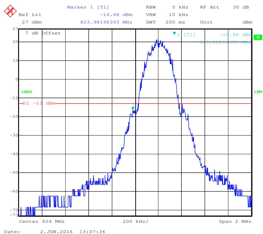
**Cellular Band, Right Band Edge for GSM (GMSK) Mode**
