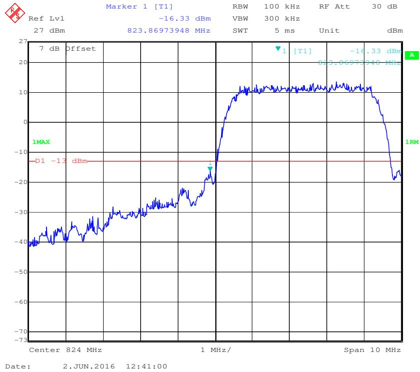
**Cellular Band, Right Band Edge for HSDPA (16QAM) Mode**
