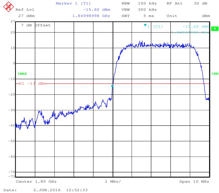
**PCS Band, Right Band Edge for WCDMA (BPSK) Mode**
