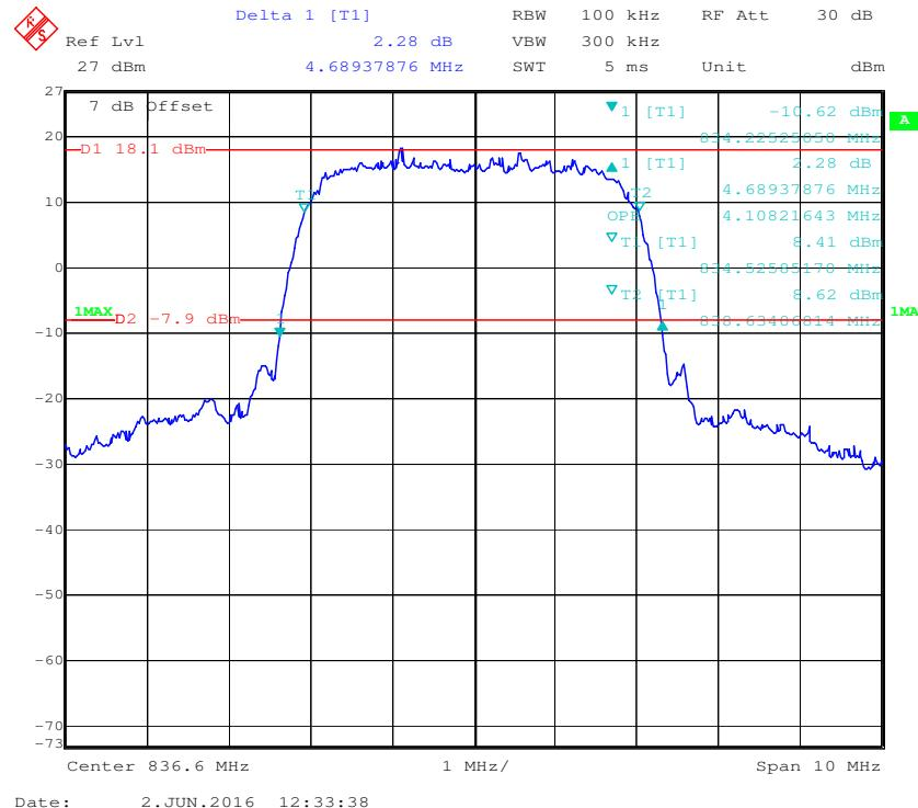
**99% Occupied&26 dB Emissions Bandwidth for HSUPA (BPSK) Mode**
