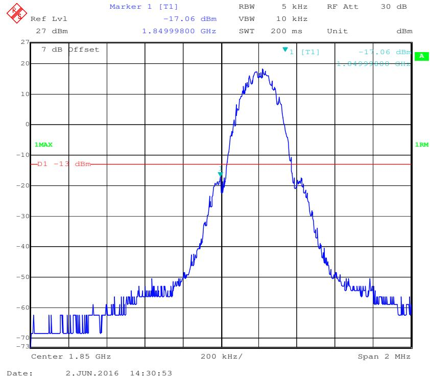
**PCS Band, Right Band Edge for GSM (GMSK) Mode**
