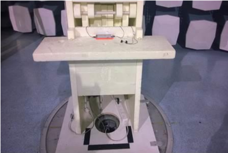
Picture 2. FCC Part 15B Radiated emissions
