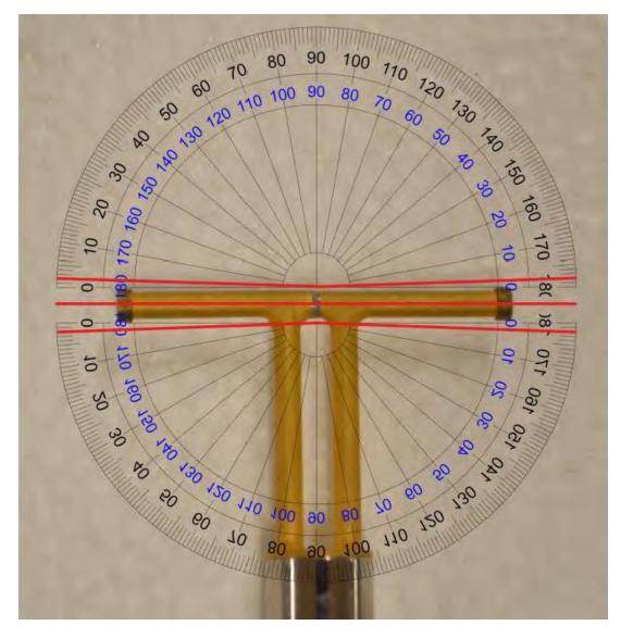
• The center red line indicates that the arms of the dipole fall within  $\pm 2^{\circ}$
