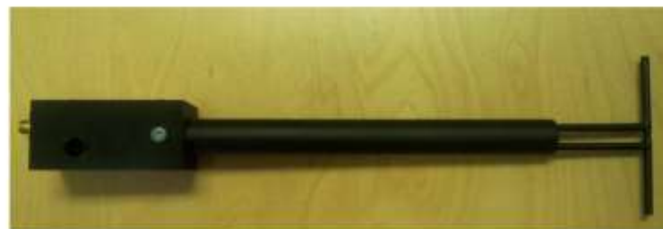
Figure 1 – MVG COMOSAR Validation Dipole
