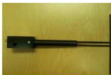
Figure 1 – MVG COMOSAR Validation Dipole
