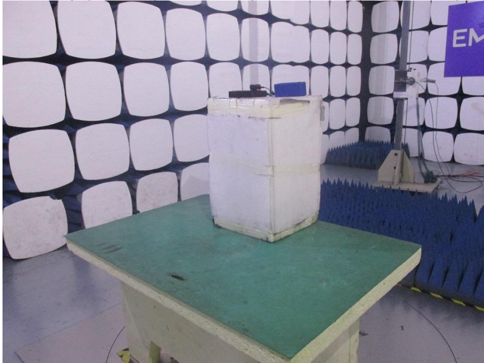
Photograph 4: Set-up for Radiated Spurious Emission above 18GHz
