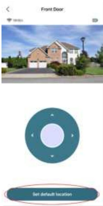
In order to ensure the effective detection of the camera and avoid missing alarms, please set the default monitoring position first. After the default monitoring position is set, the camera will automatically return to the default position after moving or rotating the PTZ.
