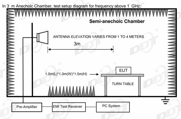
Note: For harmonic emissions test an appropriate high pass filter was inserted in the input port of AMP.
