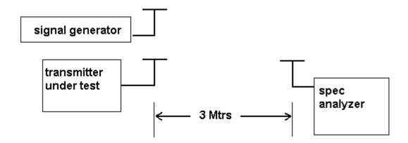
**METHOD OF MEASUREMENT:** The tabulated data shows the results of the radiated field strength emissions test. The spectrum was scanned from 30 MHz to at least the tenth harmonic of the fundamental. This test was conducted per TIA/EIA STANDARD 603 using the substitution method. Measurements were made at the test site of TIMCO ENGINEERING, INC. located at 849 NW State Road 45, Newberry, FL 32669.
