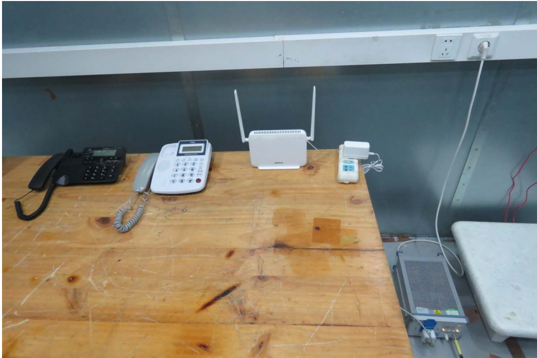
Picture 2 Conducted Emission Test Setup
