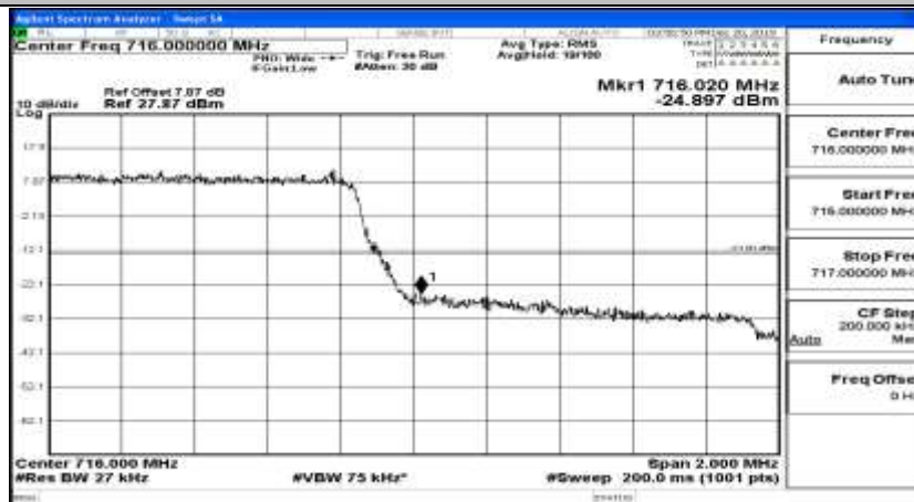
Band Edge Test Graph(s) (Channel Bandwidth: 1.4 MHz)_HCH_QPSK
