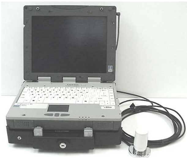
Photograph A.1-3 - DUT in Vehicle Cradle with Vehicle-Mount Antenna - front
