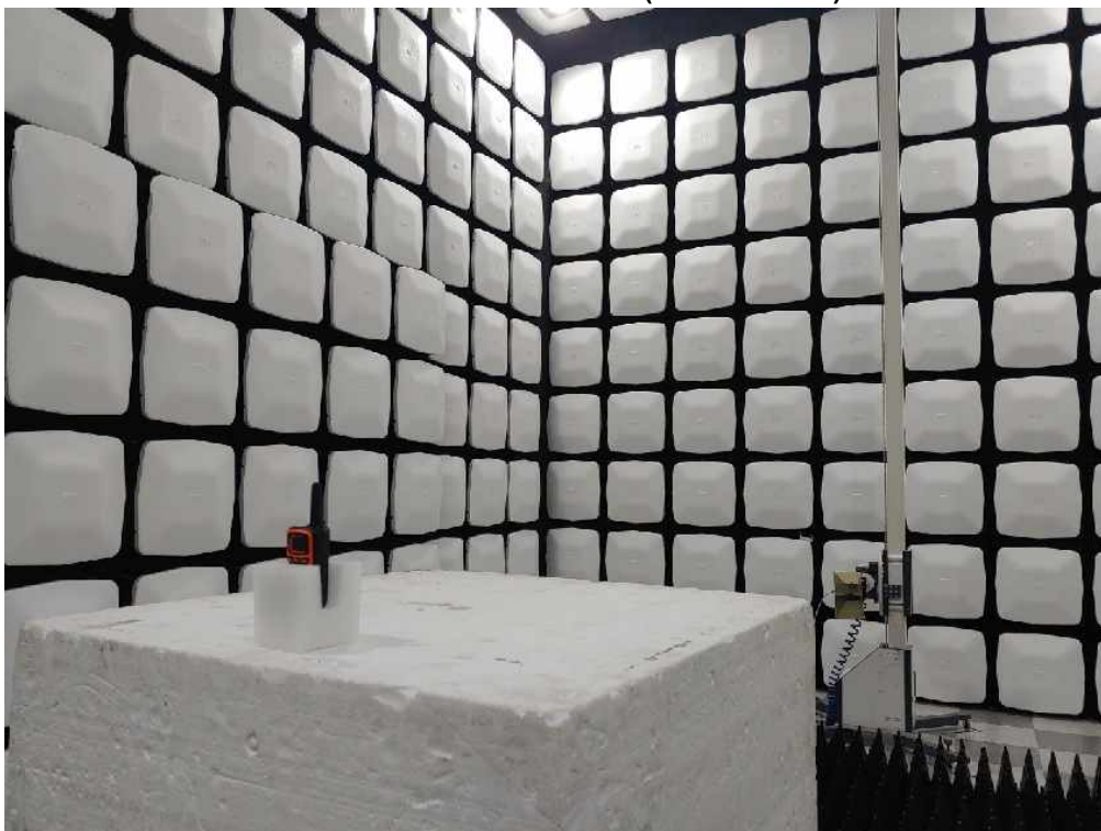
Radiated RF measurement(Above 1 GHz)
