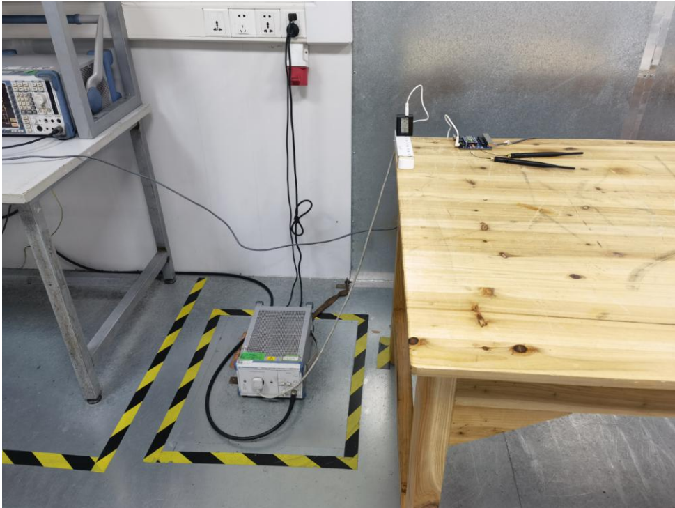
Cylindrical antenna Photo of Conducted Emission Measurement
