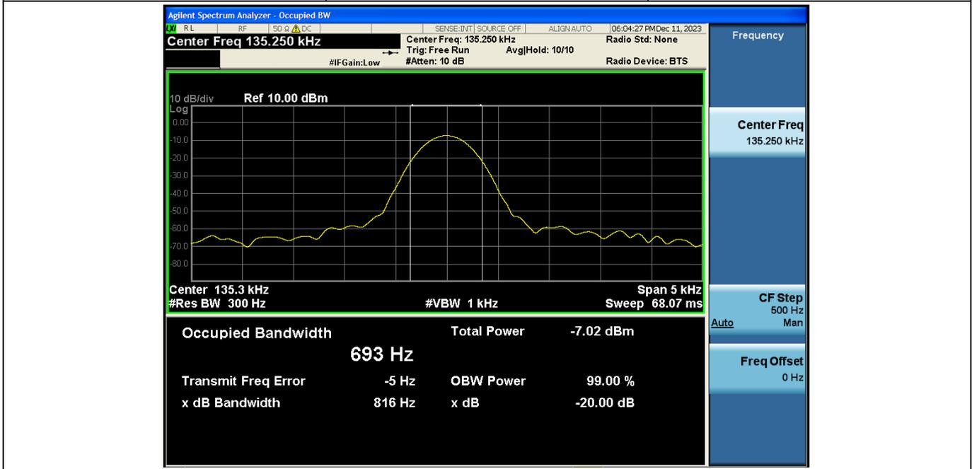
**Note:** Because the measured signal is CW-like, adjusting the RBW per C63.10 would not be practical since measurement bandwidth will always follow the RBW. The RBW is set to 300 Hz to perform the occupied bandwidth test.
