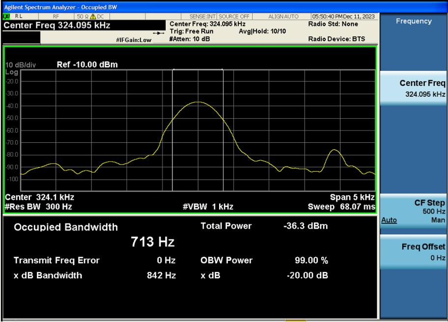
The screenshot shows the Agilent Spectrum Analyzer interface for an Occupied Bandwidth (OBW) test. The center frequency is 324.095 kHz. The occupied bandwidth is 713 Hz, and the total power is -36.3 dBm. The resolution bandwidth (RBW) is 300 Hz, and the video bandwidth (VBW) is 1 kHz. The span is 5 kHz, and the sweep time is 68.07 ms. The reference level is -10.00 dBm. The interface also shows the transmit frequency error is 0 Hz and the OBW power is 99.00%.
