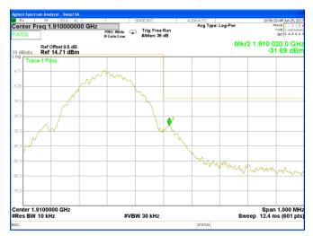
A8 FIELD STRENGTH OF SPURIOUS RADIATION MEASUREMENT GSM 850: (30-9000)MHz
