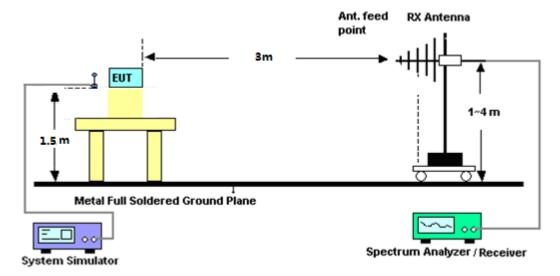
For radiated test from above 1GHz
