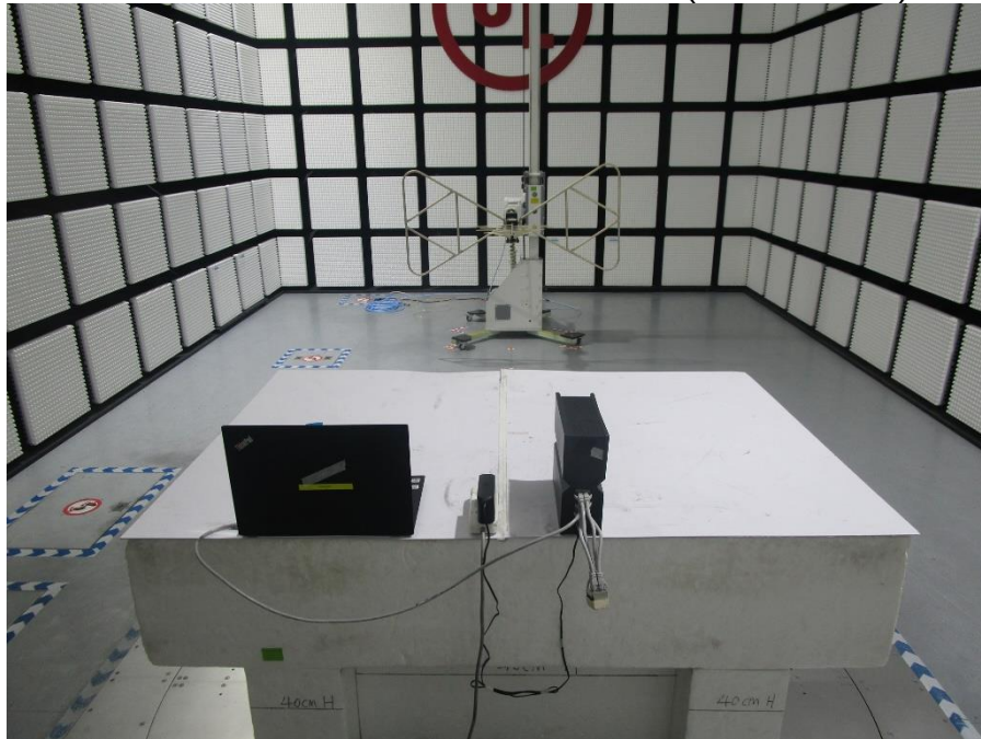
POWERLINE CONDUCTED EMISSIONS MEASUREMENT SETUP
