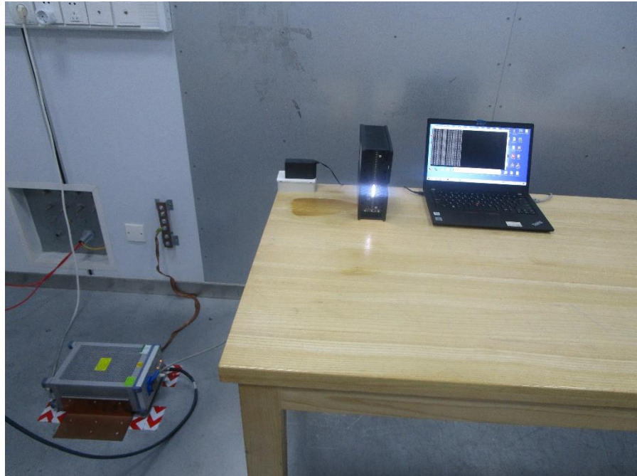
POWERLINE CONDUCTED EMISSIONS MEASUREMENT SETUP
