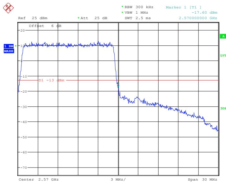
**16-QAM (15.0 MHz, FULL RB) - Left Band Edge**
