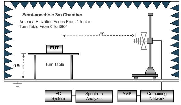
(C) Radiated Emission Test-Up Frequency Above 1GHz
