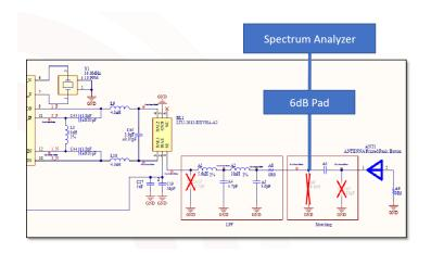
A3 is removed and a very short semi-ridged SMA coax is soldered to the A3 pad that shares a node with A6 and A8. The 6dB pad is added to present a 50 ohm termination close to the tap point. The Spectrum Analyzer is set to Max Hold and the commands from slide 8 are issued to the DUT to gather the measurement.
