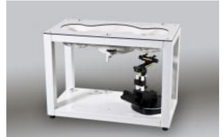
Figure 3.6 SAM Twin Phantom
