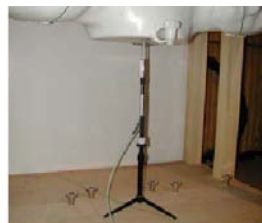
Figure 11.1 Dipole Verification Test Setup Diagram & Photo
