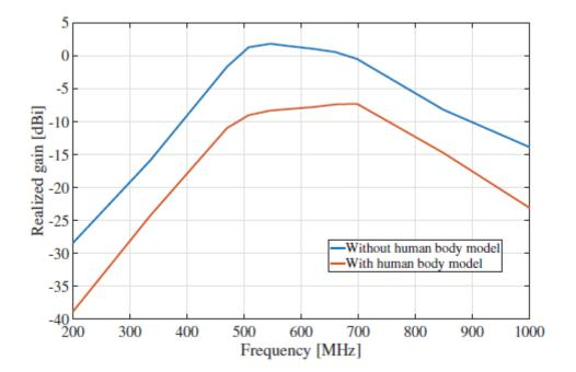
4. Maximum realized gain for the low-band monopole without the human body
