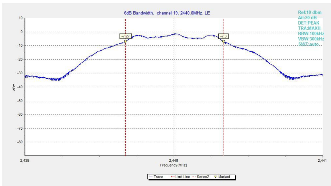
Fig.21. 6dB Bandwidth: GFSK, 2440 MHz
