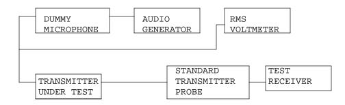
1. The test receiver audio bandwidth was <50Hz to >20,000Hz.
