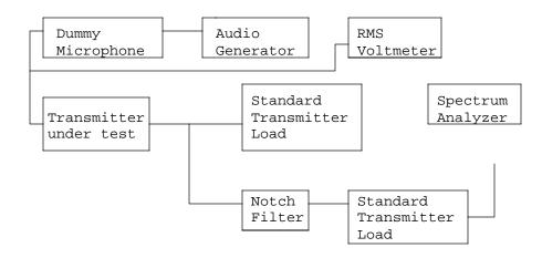
Method of Measuring Conducted Spurious Emissions
