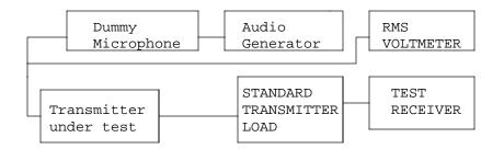
2.1051 Spurious emissions at antenna terminals(conducted): The following data shows the level of conducted spurious responses at the antenna terminal. The test procedure used was TIA/EIA 603 S2.2.13 with the exception that the emissions were recorded in dBc. The spectrum was scanned from 0.4 to at least the 10th harmonic of the fundamental.
