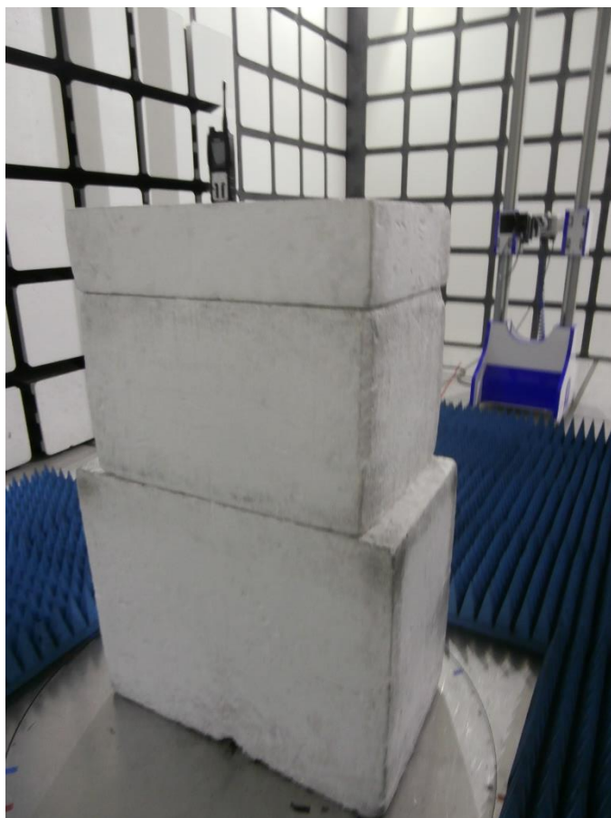
Figure 99 – Radiated Emission Setup, EUT Orientation Z
