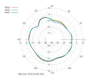
Rad #1: Dagami\_RadPatt\_Antenna gain\_#1\_Tx\_CH05\_V-YZ\_0\_CORR Rad #2: Dagami\_RadPatt\_Antenna gain\_#1\_Tx\_CH44\_V-YZ\_0\_CORR Rad #3: Dagami\_RadPatt\_Antenna gain\_#1\_Tx\_CH74\_V-YZ\_0\_CORR
