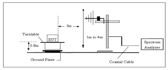
(A) Radiated Emission Test-Up Frequency 30MHz~1GHz
