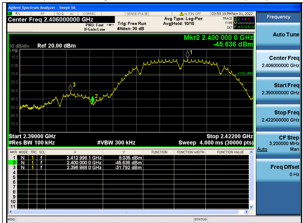
Test_Graph_802.11b_ANT1_2412_1Mbps_Lower Band Edge Emissions
