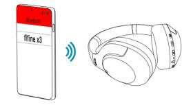
2. Turning off the headphones, press and hold the Power button for at least 5 seconds to turn on the headphones again and enter multi-point pairing mode, then pair the headphones with the second device
