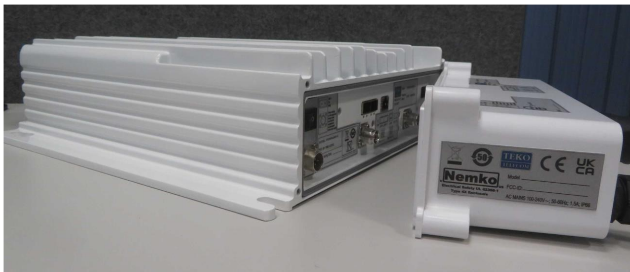
Cellhub Radio Remote Unit with optional Protection Kit
