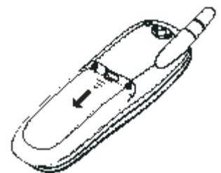
3. Insert the battery into the compartment of the phone. Place the cord between the phone body and the battery.
