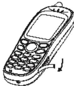
Plug the modem to the data communication port on the handset.
