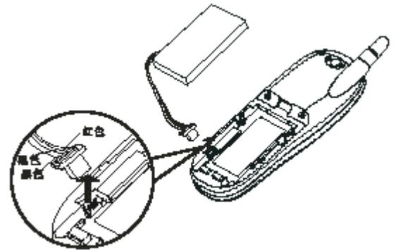
4. Connect the cord of the new battery by firmly inserting the connector until a click is heard. Check the orientation of the connector before inserting.
