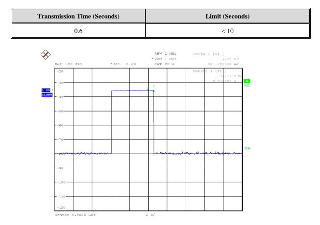
Note: The cease of transmission function operates the same way on all channels of this device. Therefore, only channel 6 was selected for testing.
