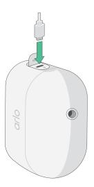
3. Connect the other end of the charging cable to a USB charging source such as a USB charging port or an AC power adapter.
