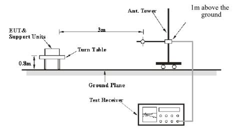
For 9kHz-30MHz test, the lowest height of the magnetic antenna shall be 1 m above the ground and three antenna orientations (parallel, perpendicular, and ground-parallel) shall be measured.
