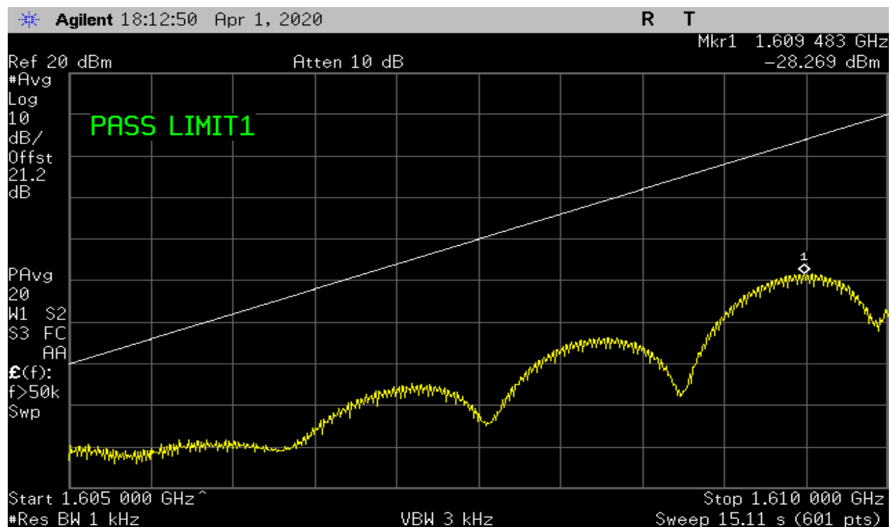
Plot 22-High Channel – Test Limit 25.216 (f)(g) – Discrete Emissions
