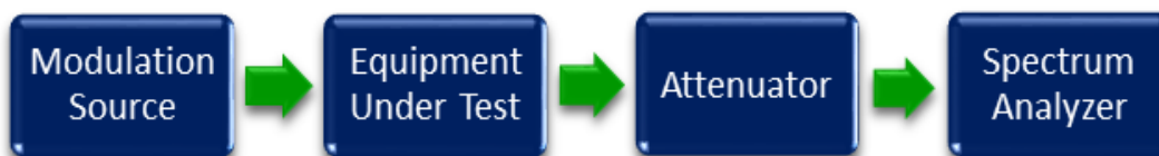
Figure 2: Occupied Bandwidth Test Setup
