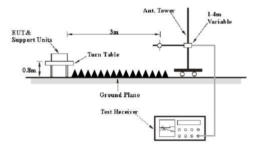
The radiated emission tests were performed in the 3 meters chamber test site, using the setup accordance with the ANSI C63.4-2014. The specification used was the FCC Part 15.109 Class B limits.
