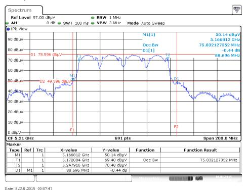
26dB Bandwidth and 99% Occupied Bandwidth Plot on Configuration IEEE 802.11ac MCS0/Nss1 VHT80 / Chain 3 + Chain 4 / 5775 MHz
