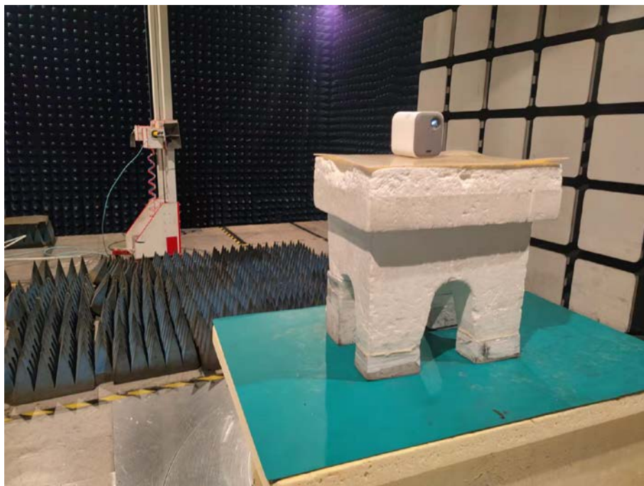
Spurious Emission Test Setup (Above 1GHz)
