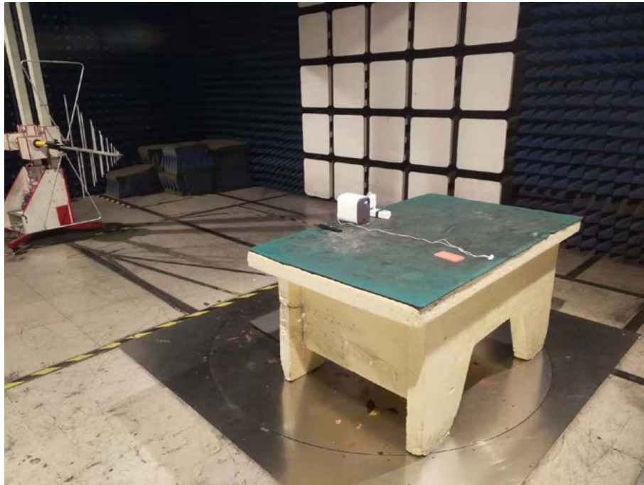
Spurious Emission Test Setup (Below 1GHz)
