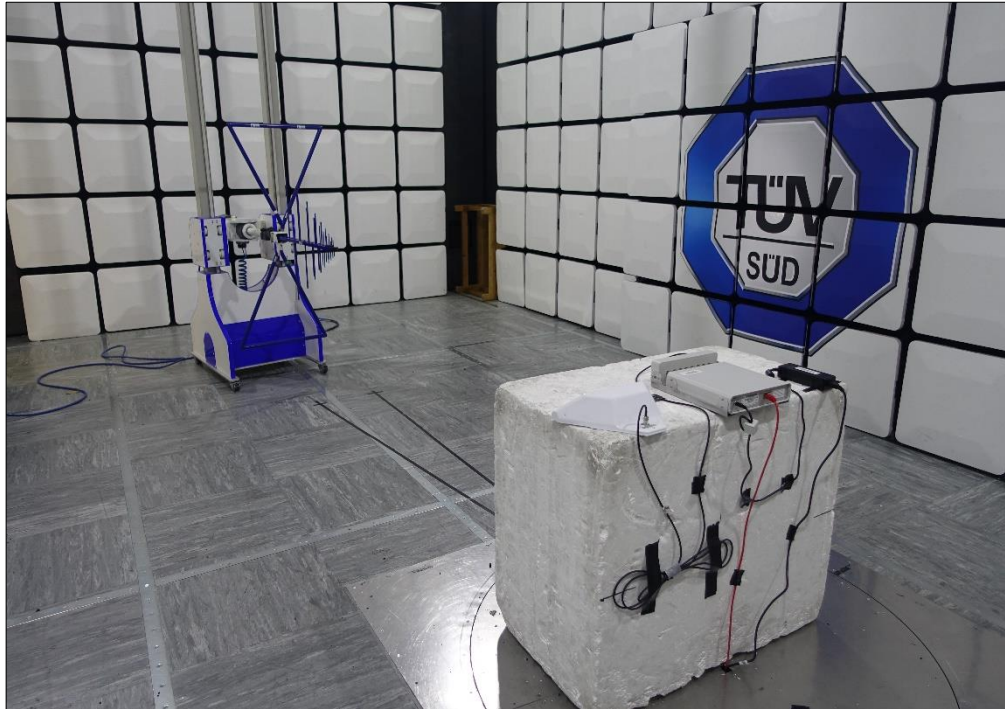
Figure 17 - Test Setup - 30 MHz to 1 GHz
