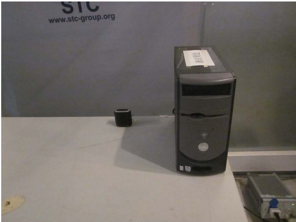
Measurement of Conducted Emission Test Set Up
