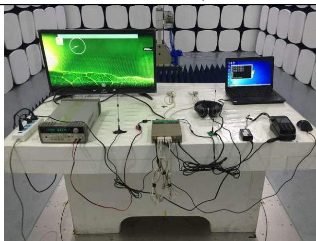
Radiated Spurious Emissions Test Setup Above 1GHz
