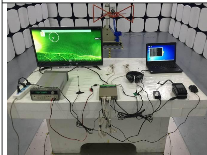
Radiated Spurious Emissions Test Setup Below 1GHz
