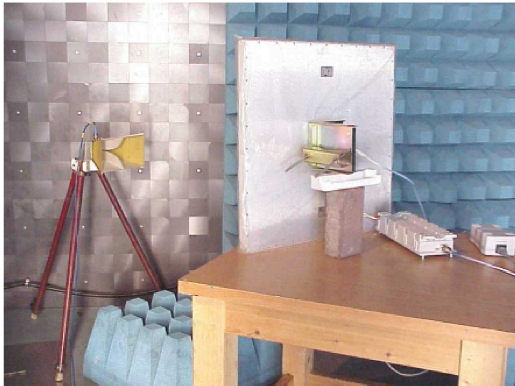
Photo #7. Radio unit with Unidirectional antenna UNI-28-4 P/N 858109 Spurious emission test
