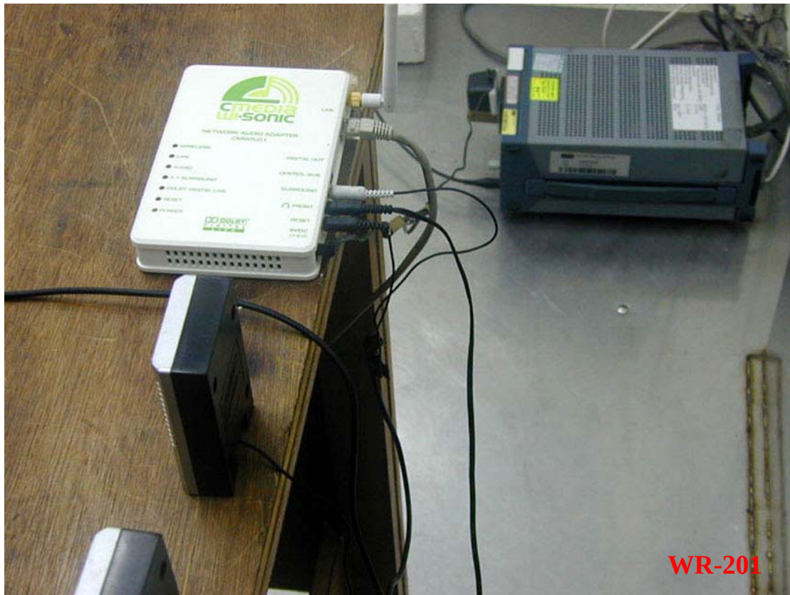
Photo 2: Conducted Emission Test Set-up photo
