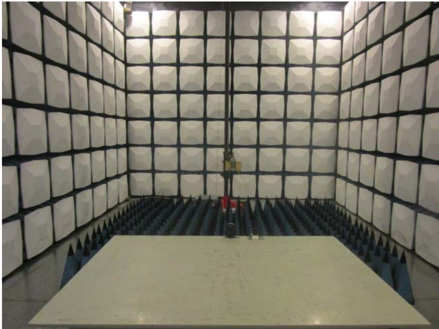
Radiated Emission - Front View (Above 1GHz)
