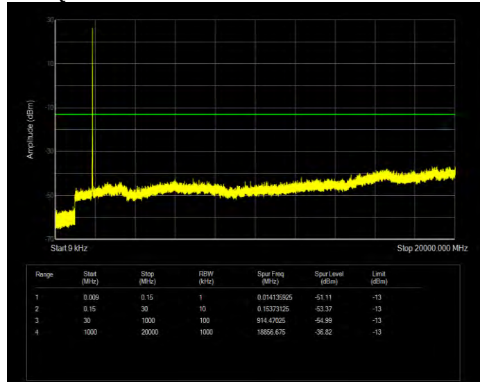
Band2 QPSK BW=5MHz Channel=19175 RB Size=1 Position=#0
