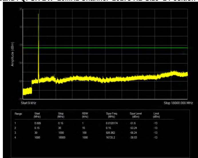
Band4 QPSK BW=20MHz Channel=20300 RB Size=1 Position=#0
