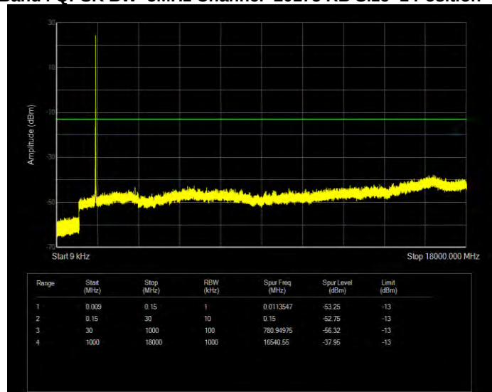
Band4 QPSK BW=5MHz Channel=20375 RB Size=1 Position=#0
