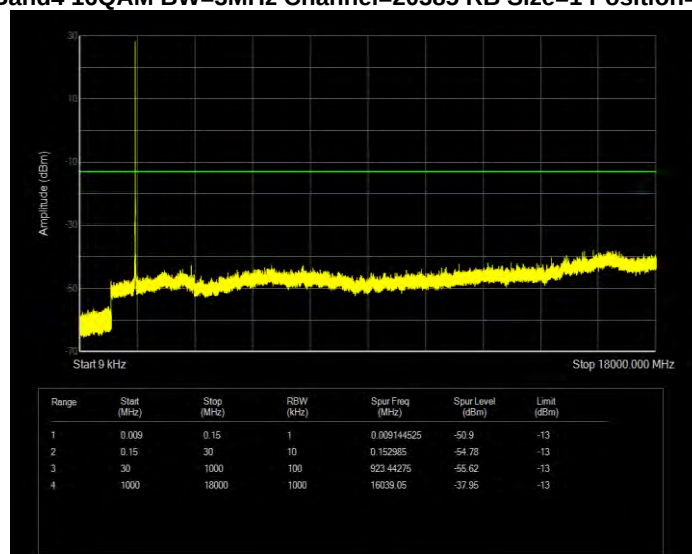
Band4 16QAM BW=5MHz Channel=19975 RB Size=1 Position=#0
