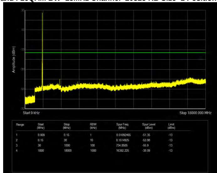
Band4 16QAM BW=20MHz Channel=20050 RB Size=1 Position=#0
