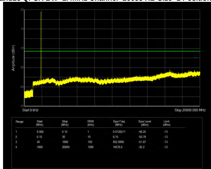
Band25 QPSK BW=10MHz Channel=26090 RB Size=1 Position=#0
