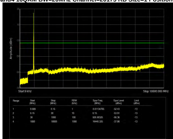
Band4 16QAM BW=20MHz Channel=20300 RB Size=1 Position=#0
