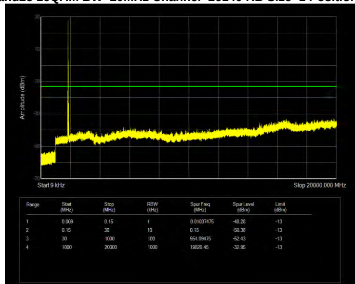
Band25 16QAM BW=20MHz Channel=26365 RB Size=1 Position=#0
