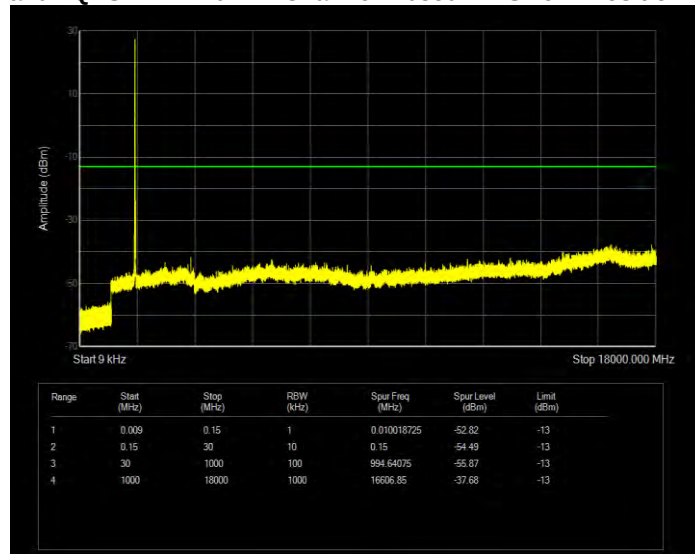
Band4 QPSK BW=15MHz Channel=20025 RB Size=1 Position=#0
