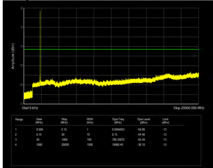
Band2 QPSK BW=3MHz Channel=19185 RB Size=1 Position=#0
