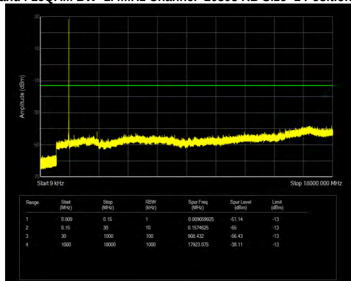
Band4 16QAM BW=10MHz Channel=20000 RB Size=1 Position=#0
