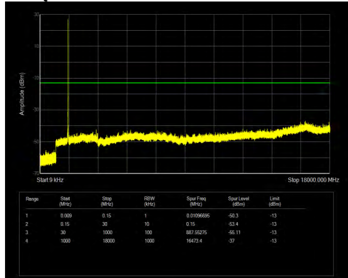
Band4 QPSK BW=5MHz Channel=19975 RB Size=1 Position=#0
