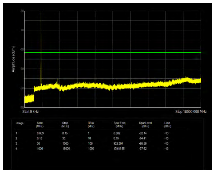
Band4 16QAM BW=5MHz Channel=20175 RB Size=1 Position=#0
