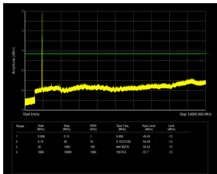
Band4 16QAM BW=10MHz Channel=20175 RB Size=1 Position=#0
