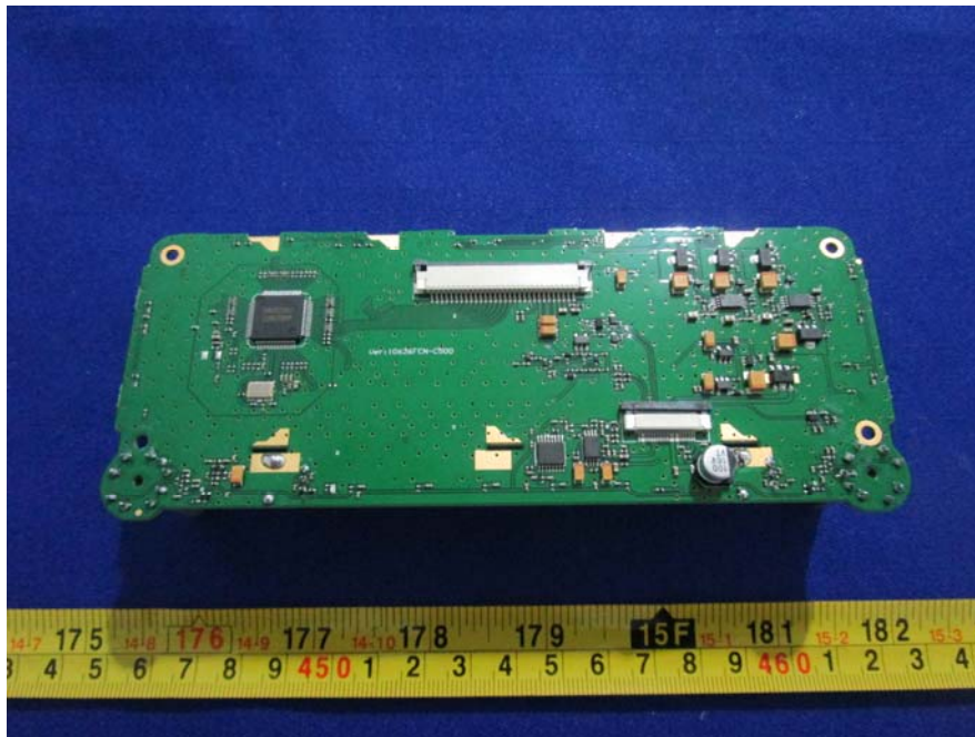
EUT –Control Panel Mainboard Bottom View
