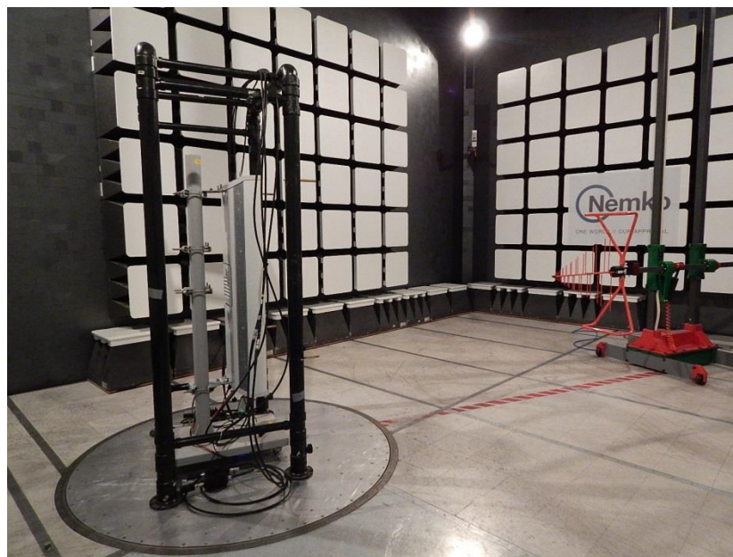
Figure 8.1-38: Setup photo – 30 to 1000 MHz
