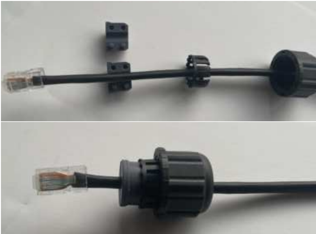
Figure 2: RJ45 Plug Assembly on IP67 cable gland
